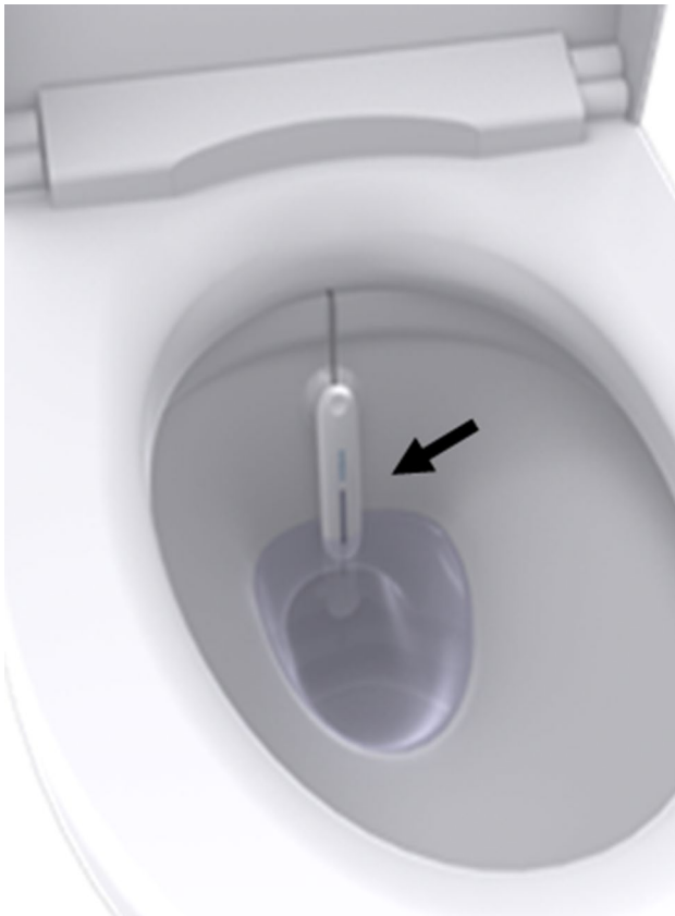
Fig. 2 The s-HMSU system includes a server, measurement device, and a user terminal. The sensor is located in the water in the toilet bowl (black arrow). s-HMSU, self-health monitoring system for urine excretion
